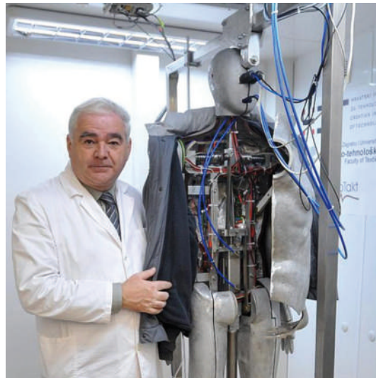
Measurement system for the determination of thermal properties of clothing, so-called thermal manikin
