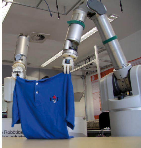
Robot grasping the cloth with mechanical gripper
