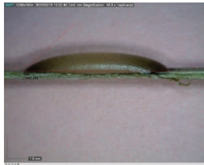
Microscopic analysis of the lateral (left) and upper (right) sides of cured droplets resin on highly oriented roving yarns
