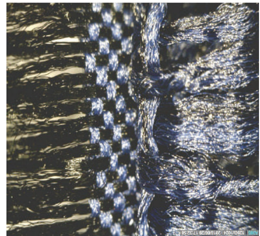
Cross section of multilayer interlacing woven fabric
