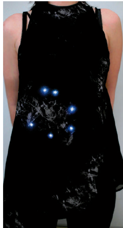
E-clothing garment with integrated LEDs
