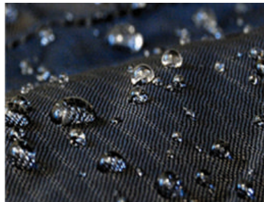
Plasma treatment of textiles with hydrophobic and antimicrobial properties
