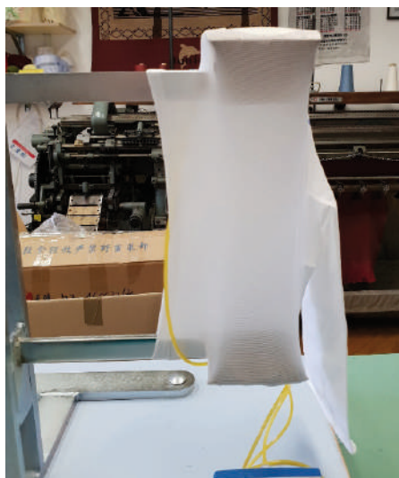
Compressional scissors for measuring compressibility of tubular elastic knitwear
