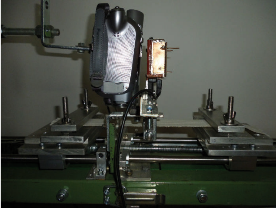
Measuring system for measurement of fabric thickness
