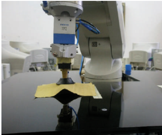
Grasping textile materials with a vacuum gripper
