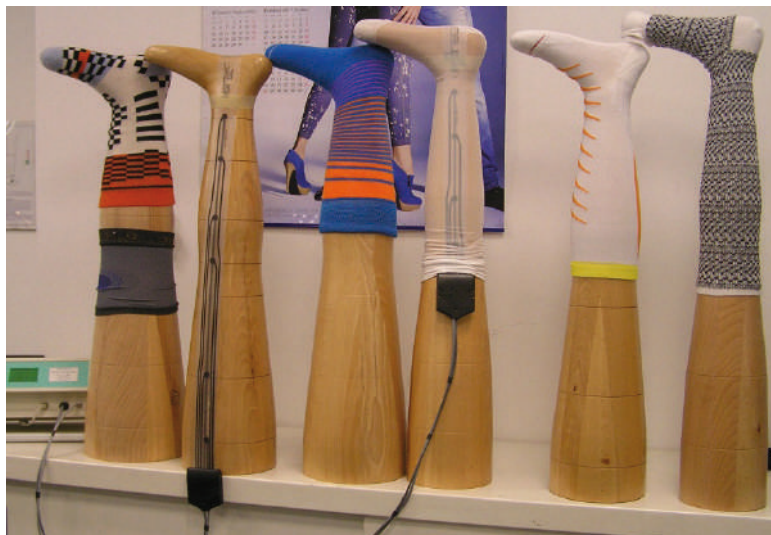
Wooden leg models for measuring compressibility of hosiery
