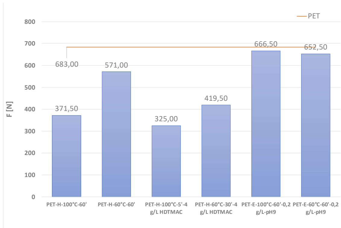
Figure 2: Breaking force (F) before (PET) and after hydrolysis of PET fabrics
