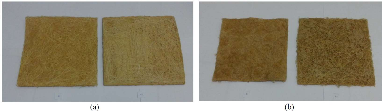
FIGURE 2. (a) Composite from raw CHF: latex = 30:70 (left) and 50:50 (right), (b) composite from CHF treated NaOH 5%: latex = 30:70 (left) and 50:50 (right)
